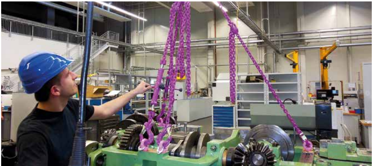
ICE 120 – 13mm WLL 8.0t 1 Metre = 4.25kg
