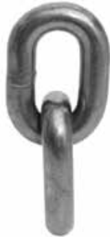
Grade 80 – 16mm WLL 8.0t 1 Metre = 5.65kg
