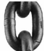
Figure 2 - location of nicks indicate the severity
