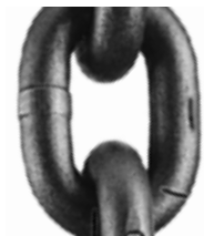
Figure 2 - location of nicks indicate the severity
