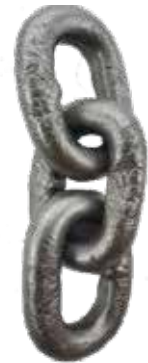
Figure 1 - nicked and gouged links
