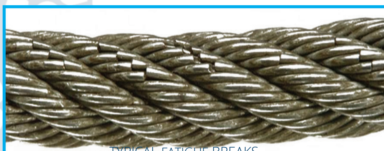
TYPICAL FATIGUE BREAKS
